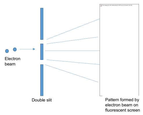
(c) The pattern formed on the fluorescent screen by the electrons as they passed through the double slit one at a time showed evidence that electrons possessed a 'wave nature'. Explain using your knowledge of wave properties.
