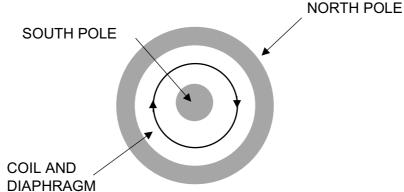
(e) At the instant that the coil is carrying a clockwise conventional current, state whether the magnetic force experienced by the coil is 'into the page' or 'out of the page'.
